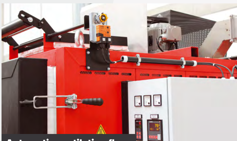
Automatic ventilation flap
