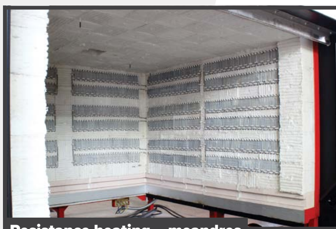
Resistance heating – meandres
